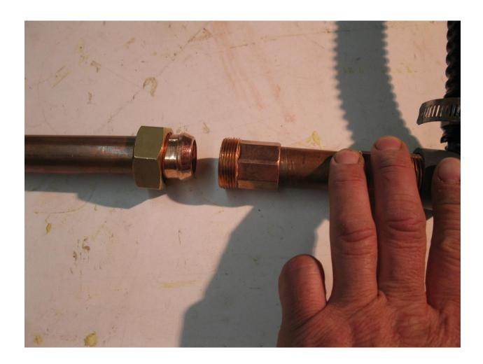
The final connections shown below. The copper tube will be mounted through a hole drilled through the center of the glazed pot.
